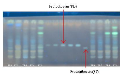
HPTLC profile of Tribulus terrestris accessions with Protodioscin (PD) & Prototribestin (PT) (after derivatization with vanillin-sulphuric acid and visualized under \lambda 366 nm)
